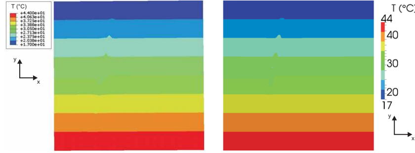
Fig. 9.2.8: Temperature (°C) calculated with ABAQUS (left) and OGS (right). Temperature increase (decrease) can be observed in the fold as a result of fluid outflow from the storage aquifer into the fault.
