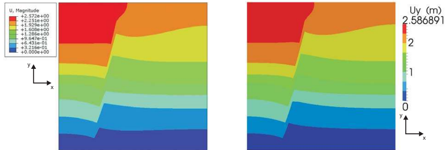
Fig. 9.2.5: : Displacement in the y direction (m) calculated with ABAQUS (left) and OGS (right)
